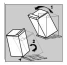
Tilt the washing machine backwards, rotate it by a quarter of a turn on one of its corner to remove the transport base.
